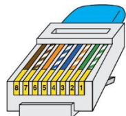
Figure 13-3 CVS module connector pinout
