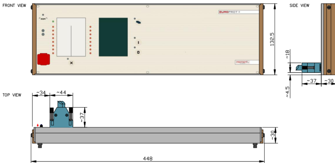
Figure 21-28 Dimensions for 84 HP wide remote HMI
