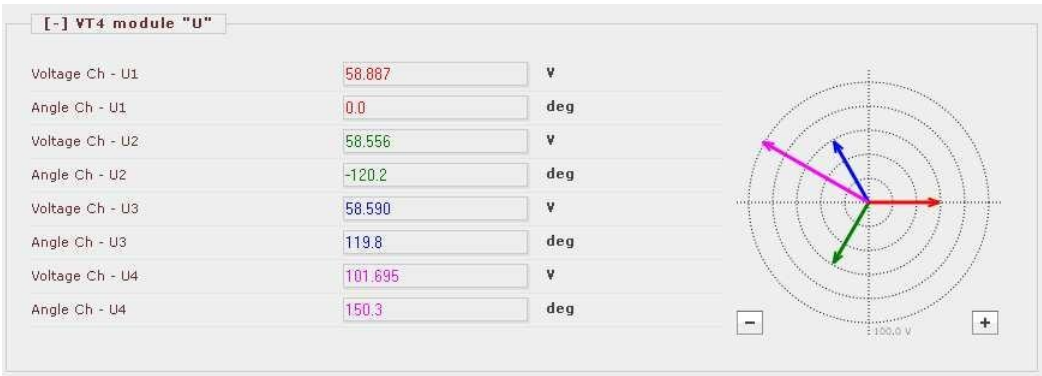
Figure 1-7 Example:On-line measurement for syncrocheck, using phase-to-phase voltage
