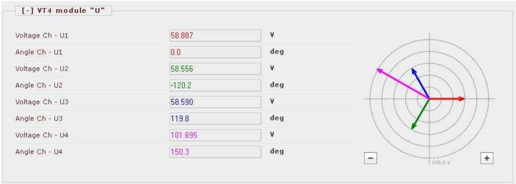
Figure 1-7 Example:On-line measurement for syncrocheck, using phase-to-phase voltage
