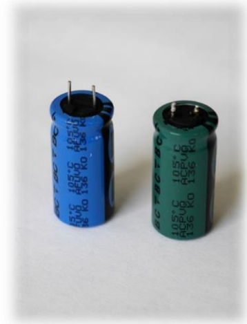
Figure 4-1 The capacitor on the right is already discolored
