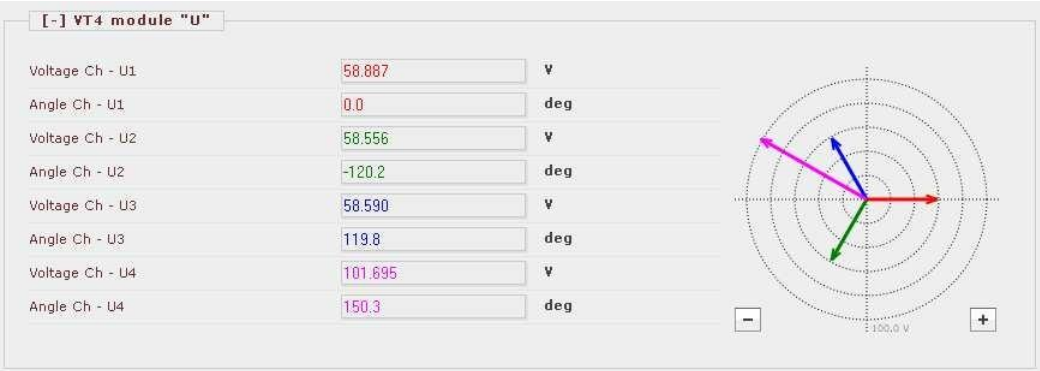
Figure 1-7 Example:On-line measurement for syncrocheck, using phase-to-phase voltage
