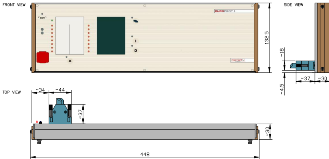
Figure 21-28 Dimensions for 84 HP wide remote HMI
