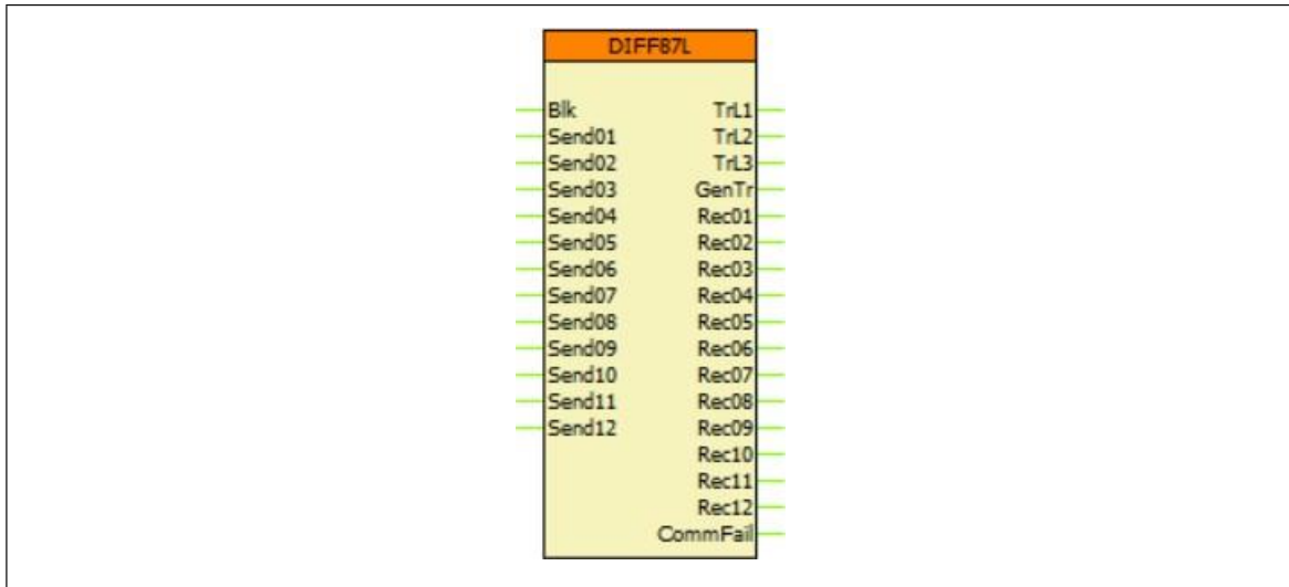
Figure 2-1 Graphic appearance of the function block of the line differential protection function for two ends
