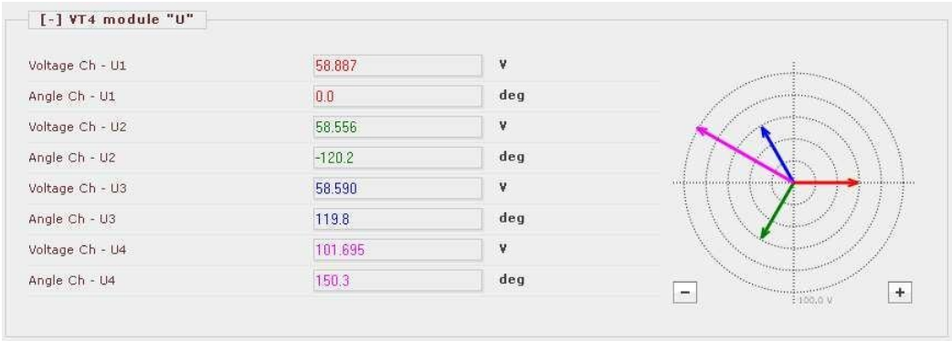
Figure 1-7 Example:On-line measurement for syncrocheck, using phase-to-phase voltage
