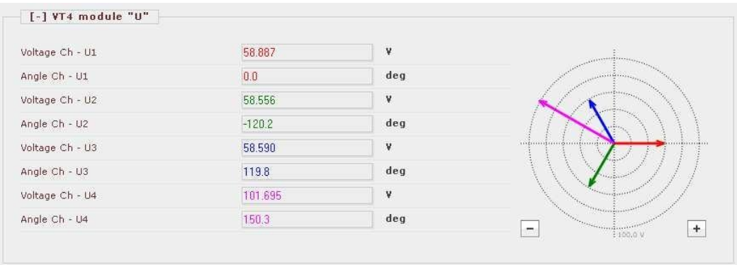
Figure 1-7 Example:On-line measurement for syncrocheck, using phase-to-phase voltage
