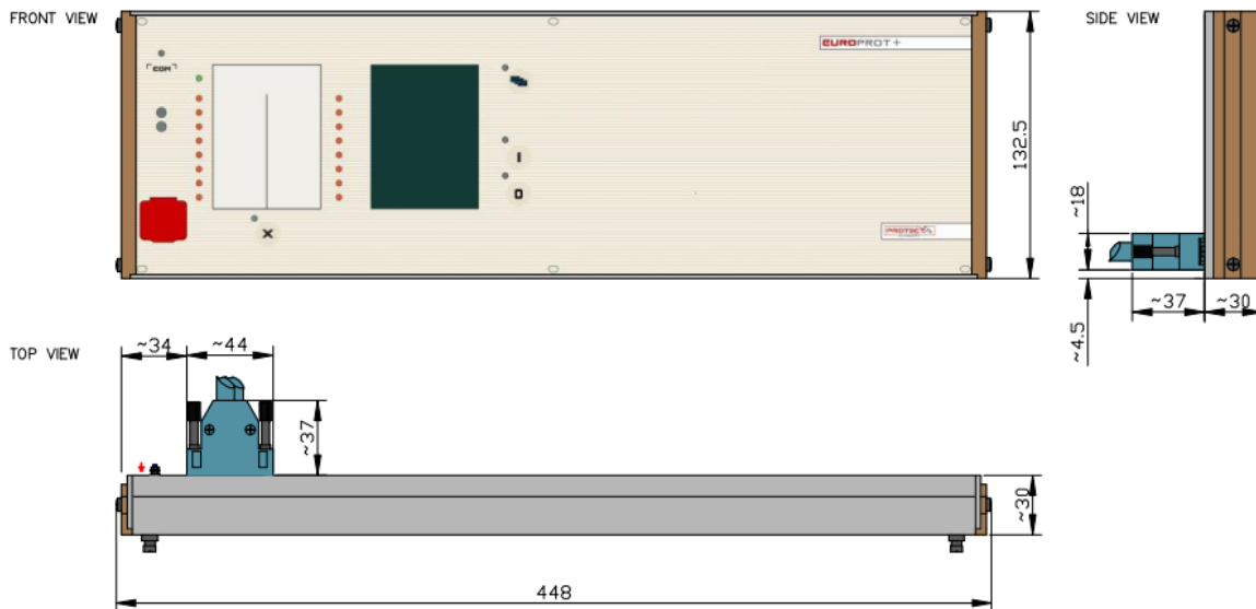
Figure 21-28 Dimensions for 84 HP wide remote HMI
