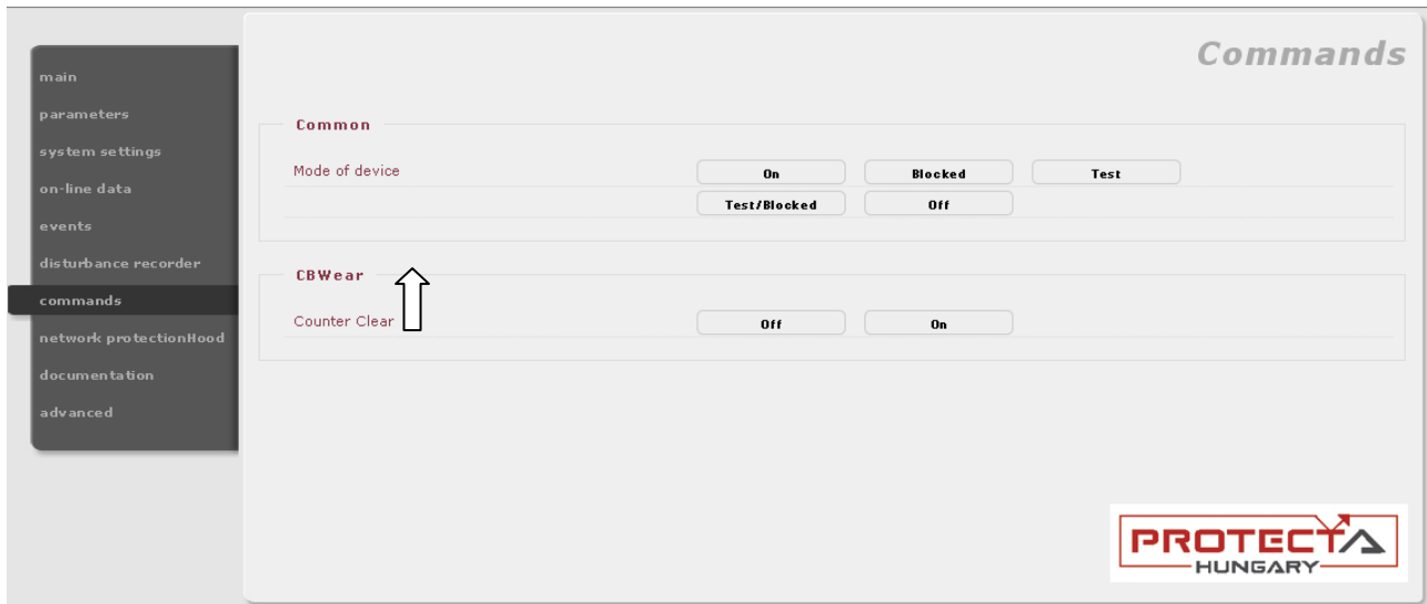
Figure 1-2 The command window to reset the CB wear counter
