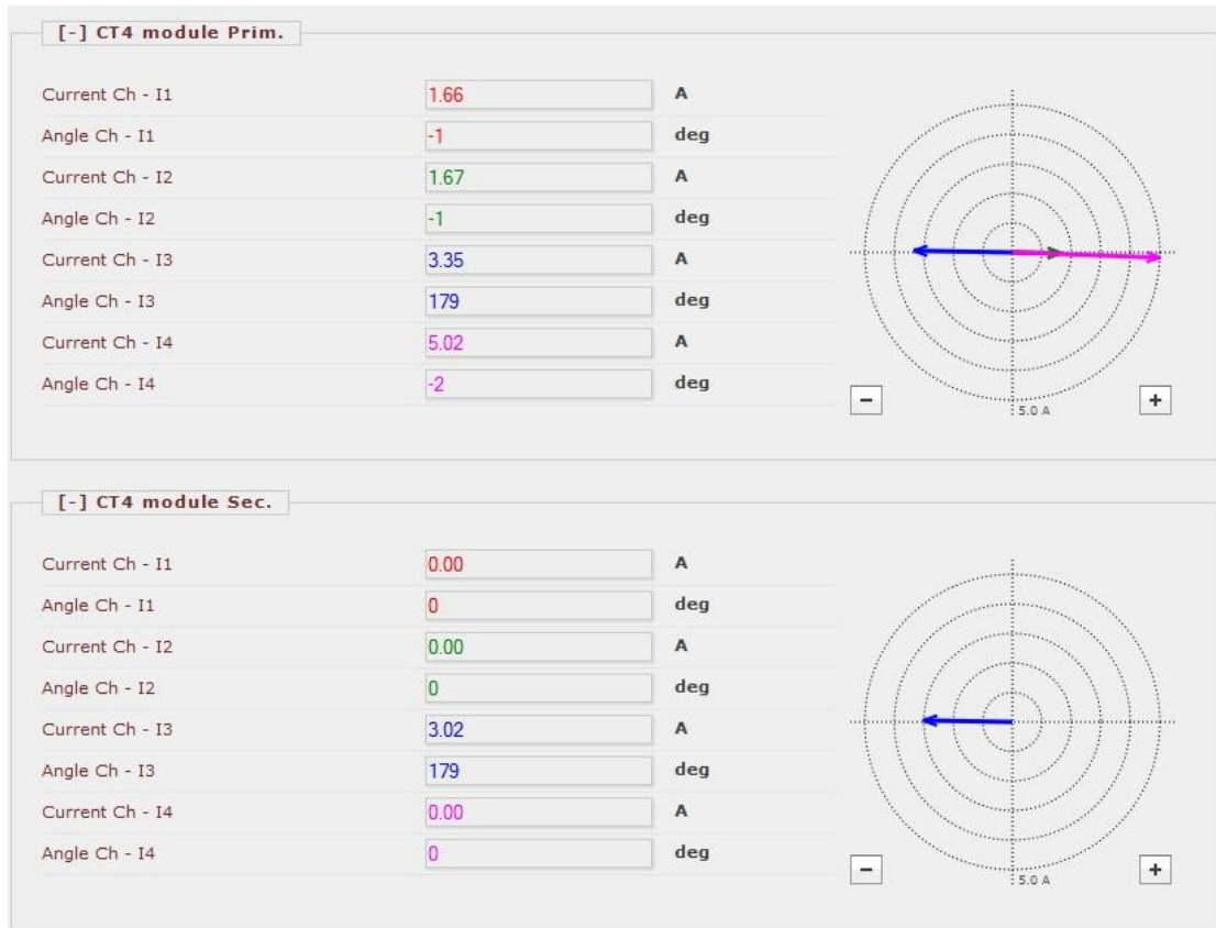
Figure 5-8 Measured currents of the CT modules
