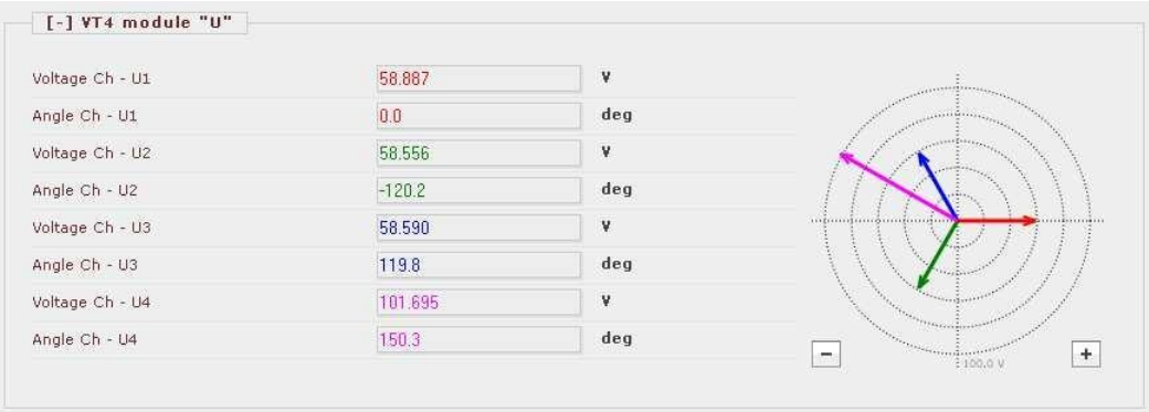
Figure 1-7 Example:On-line measurement for syncrocheck, using phase-to-phase voltage
