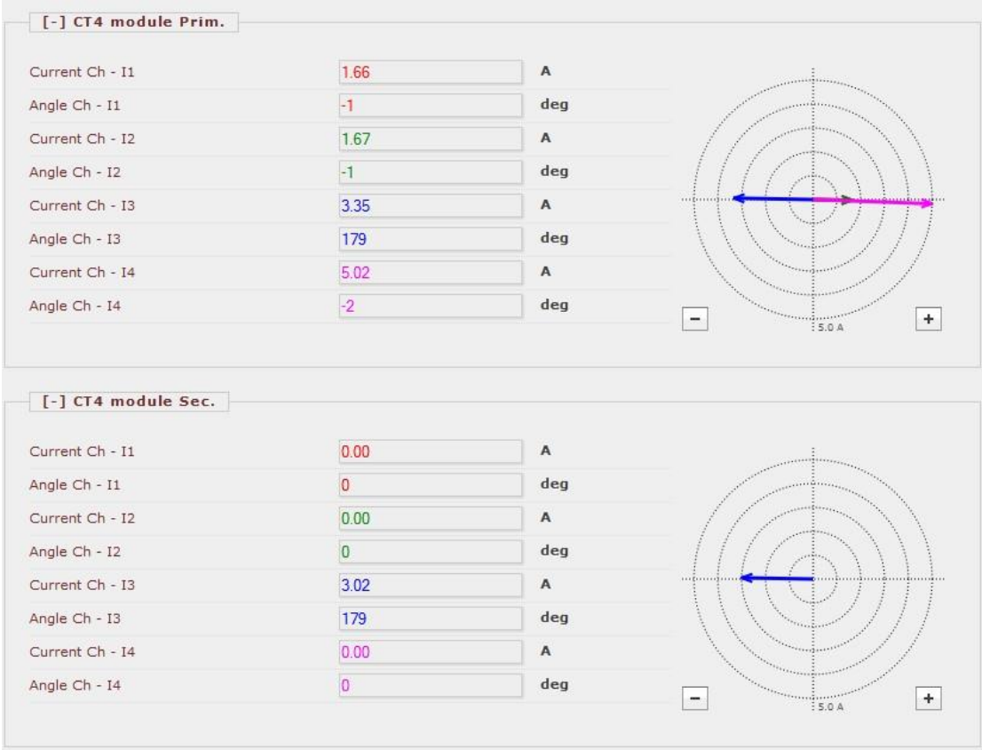
Figure 5-8 Measured currents of the CT modules
