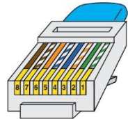
Figure 13-3 CVS module connector pinout
