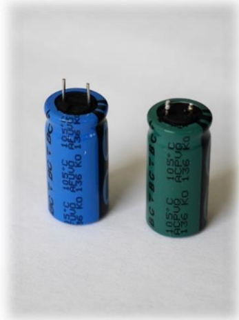
Figure 4-1 The capacitor on the right is already discolored
