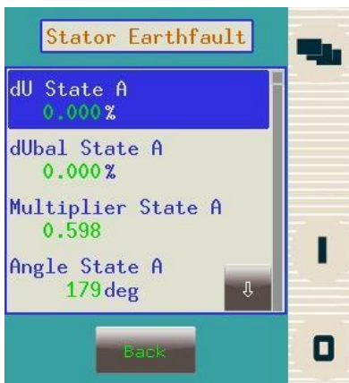
Figure 15 On-line window after balancing (No neutral grounding resistor)
