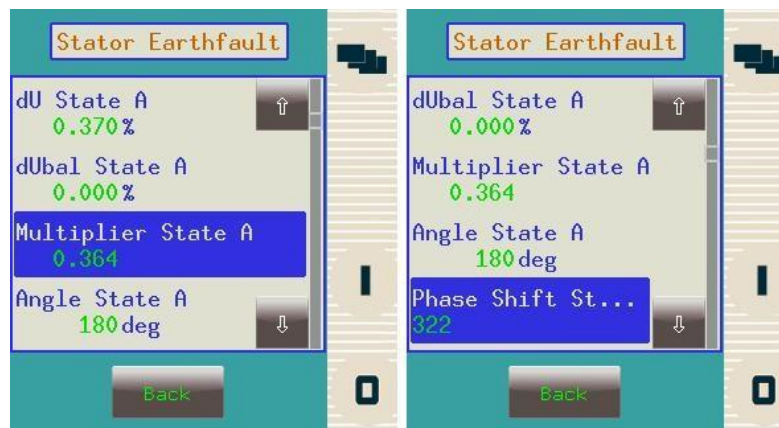
Figure 21 On-line window during balancing (With neutral grounding resistor)
