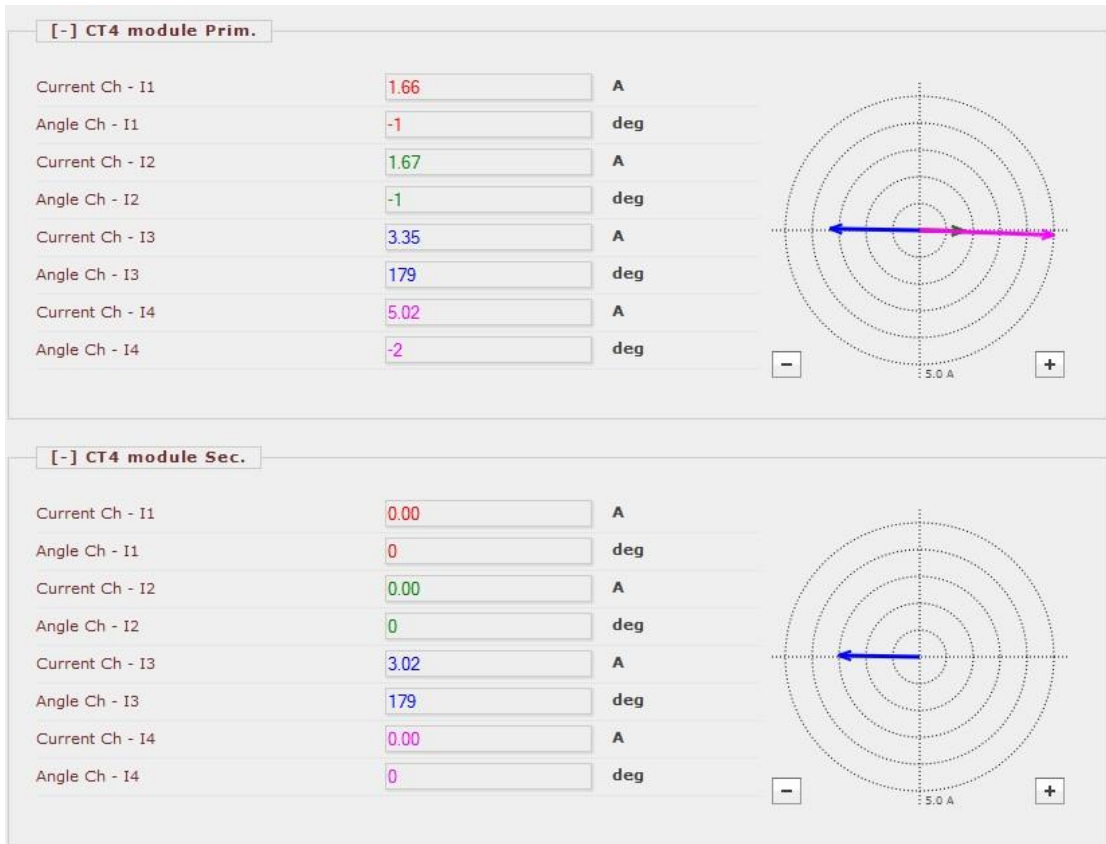
Figure 5-8 Measured currents of the CT modules
