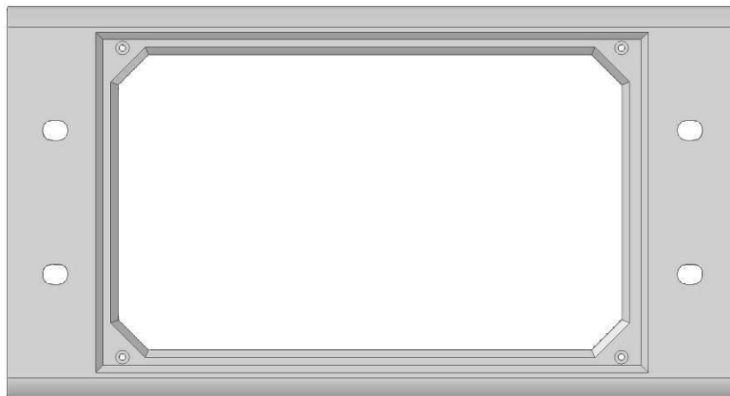
Figure 21-20 42 HP IP frame front view
