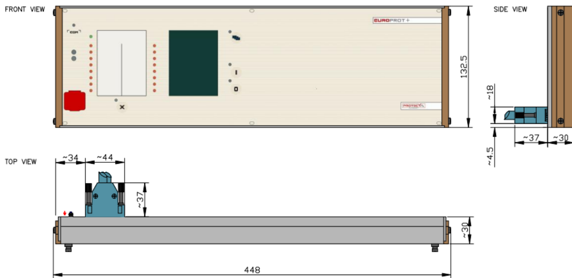
Figure 21-28 Dimensions for 84 HP wide remote HMI
