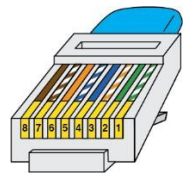
Figure 13-3 CVS module connector pinout
