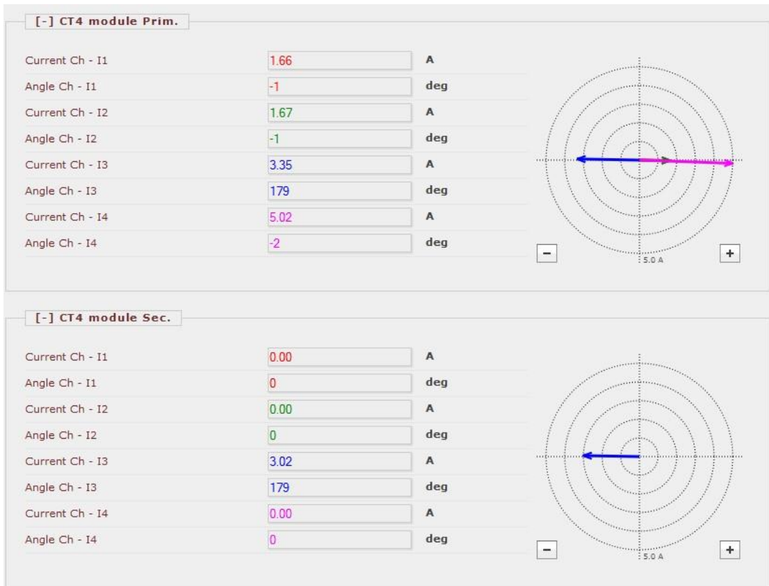
Figure 5-8 Measured currents of the CT modules
