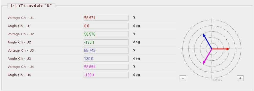
Figure 1-4 Example: On-line measurement for syncrocheck, using phase-to-neutral voltage
