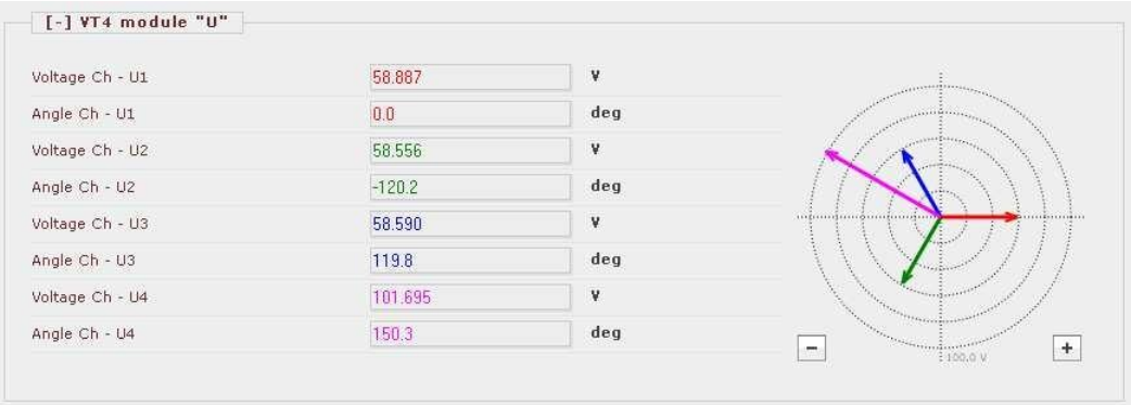
Figure 1-7 Example:On-line measurement for syncrocheck, using phase-to-phase voltage
