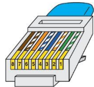
Figure 13-3 CVS module connector pinout
