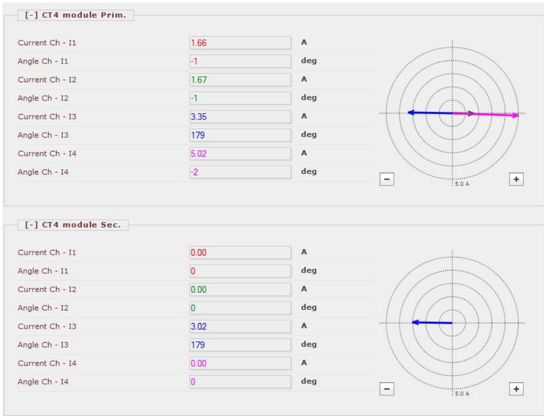
Figure 5-8 Measured currents of the CT modules
