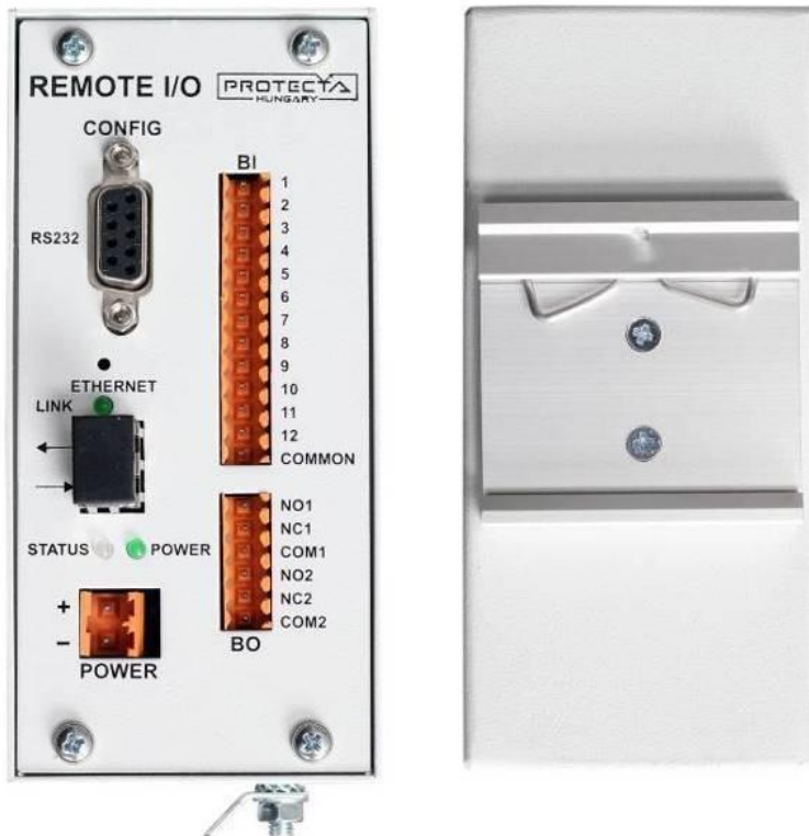
Figure 1-2 Front view and rear view with fastening for mounting rail
