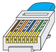
Figure 13-3 CVS module connector pinout
