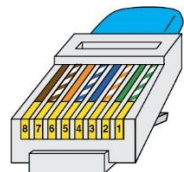
Figure 13-3 CVS module connector pinout
