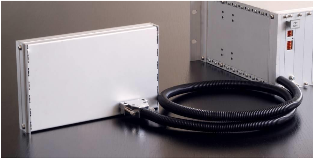
Figure 4–2 Remote HMI module with its host device
