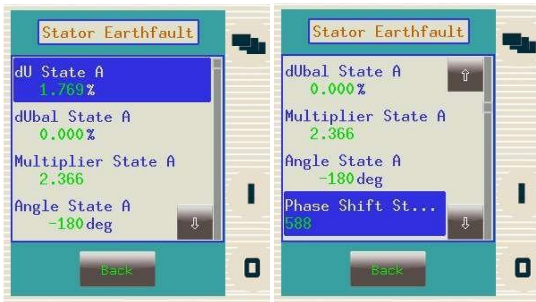
Figure 1-4 On-line screen of the device during balancing procedure
