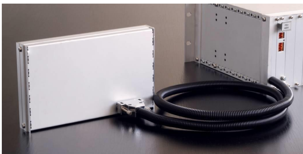
Figure 4-2 Remote HMI module with its host device
