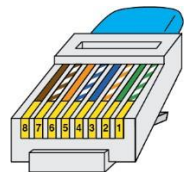
Figure 13-3 CVS module connector pinout
