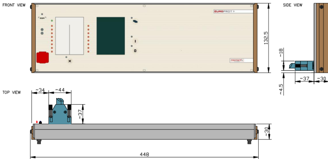
Figure 21-28 Dimensions for 84 HP wide remote HMI
