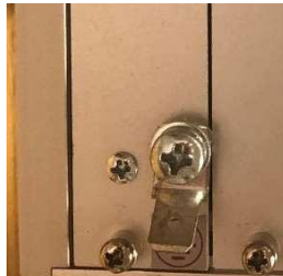
Picture 3-5-1-1 Earth connection point of the device at the Power supply module
