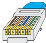
Figure 13-3 CVS module connector pinout
