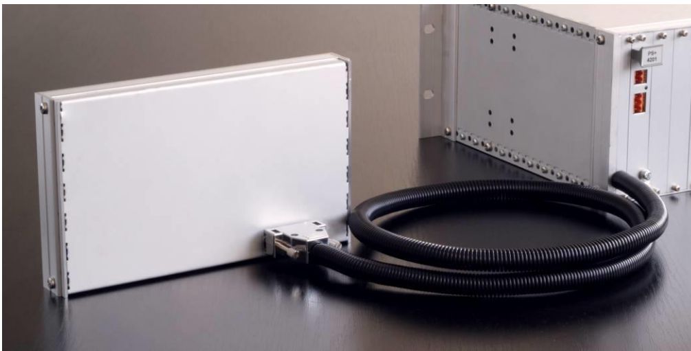
Figure 4-2 Remote HMI module with its host device
