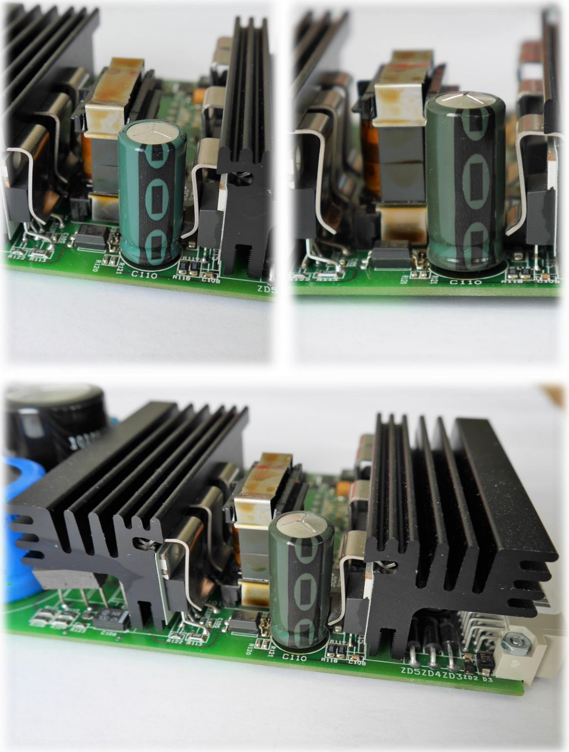
Figure 4-3 Faulty capacitances on visual inspection. The discoloration compared to the original blue color is clearly visible, bloating can be seen on 2 of them
