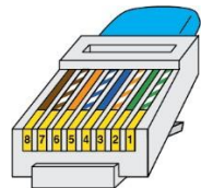
Figure 13-3 CVS module connector pinout
