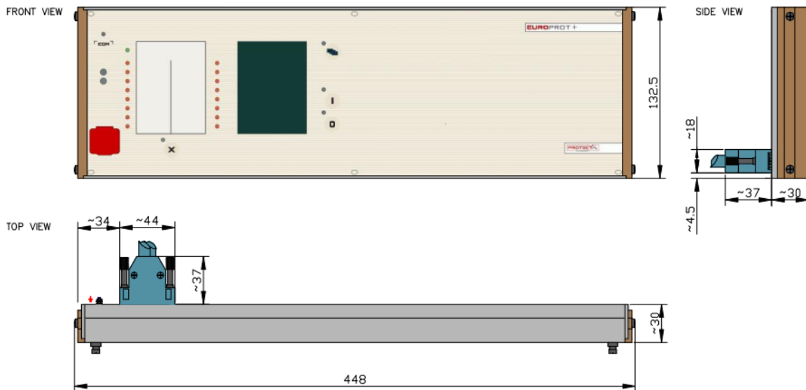
Figure 21-28 Dimensions for 84 HP wide remote HMI
