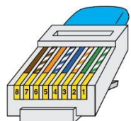
Figure 13-3 CVS module connector pinout
